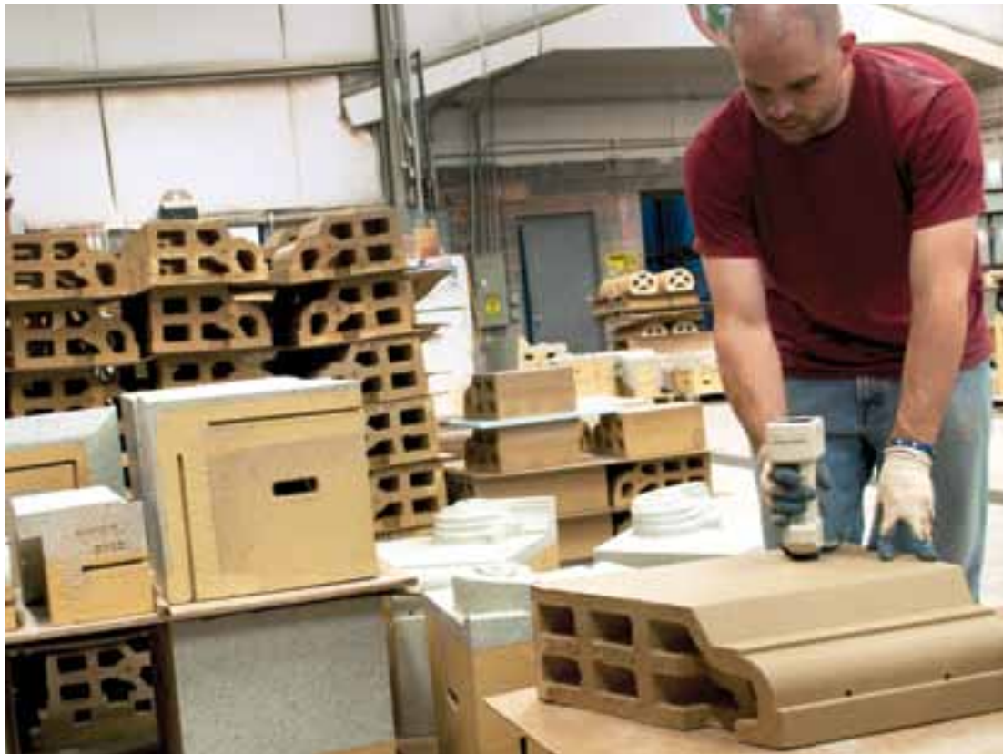
BELOW: A single color glazed unit is checked with a Spectrophotometer.
