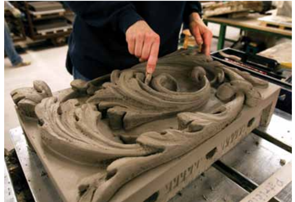
LEFT: Boston Valley created restoration pieces for Cass Gilbert's 90 West St. façade that were damaged during the September 11th attacks.
