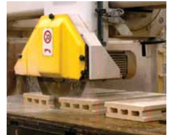
A laser-aligned, diamond-edged wet gantry saw cuts finished pieces to proper length.
