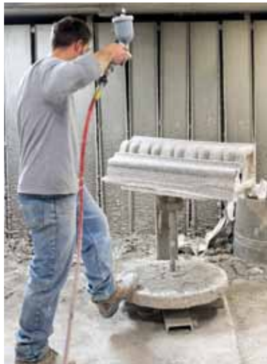
A Boston Valley craftsman applies glaze to a terra cotta unit.
